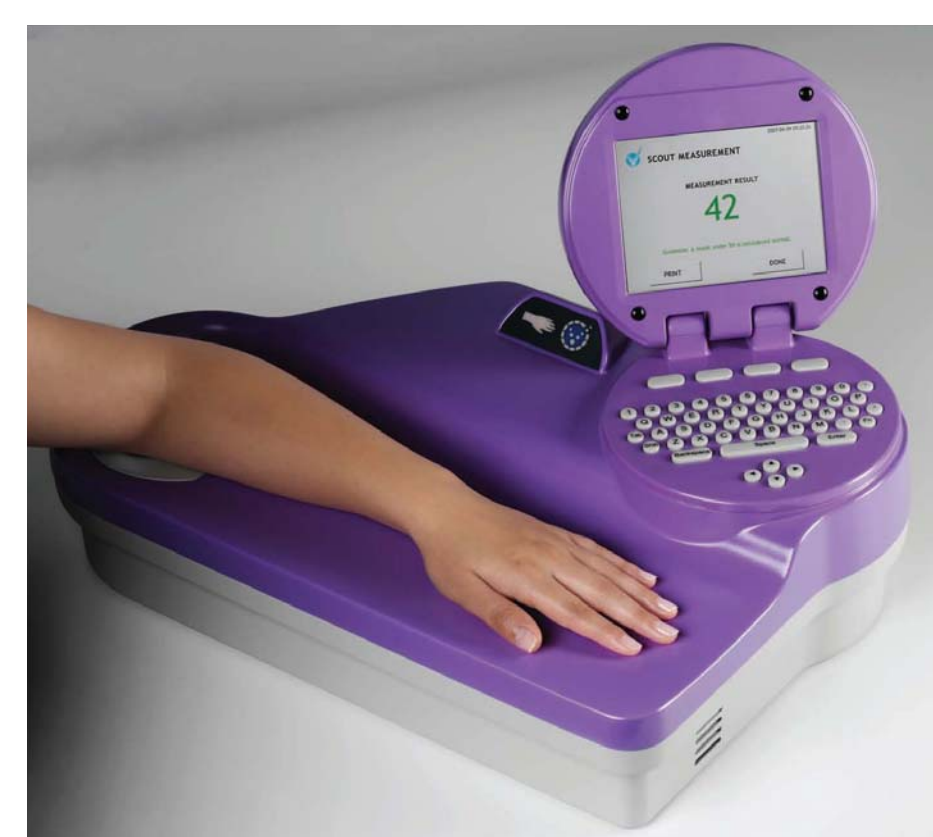
Figure 1: Noninvasive assessment of skin AGEs using a skin fluorescence spectrometer
